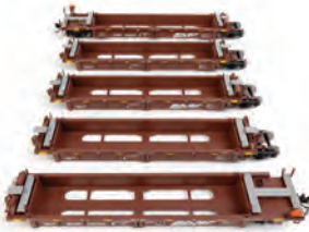
HO Thrall 5-Unit Rebuilt 40' Well Car WaltherMainline. Feature 100- and 70-ton roller bearing trucks, correct 38" and 33" turned metal wheelsets, a heavy die-cast metal frame for superb performance empty or loaded, finely molded 3-D brake rods with chains, brake piping and weld lines on body, separate deck-mounted brake detail with piping, IBC storage boxes and realistic walkways, and Proto MAX ™ metal knuckle couplers. BNSF Railway 910-55660 #238140 A-E 910-55661 #238175 A-E 910-55662 #238212 A-E 910-55663 #238223 A-E Reg. Price: $149.98 Sale: $120.98
