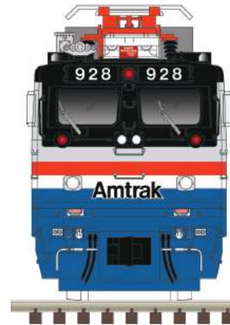
Amtrak end shown with Amtrak-style ditchlights
